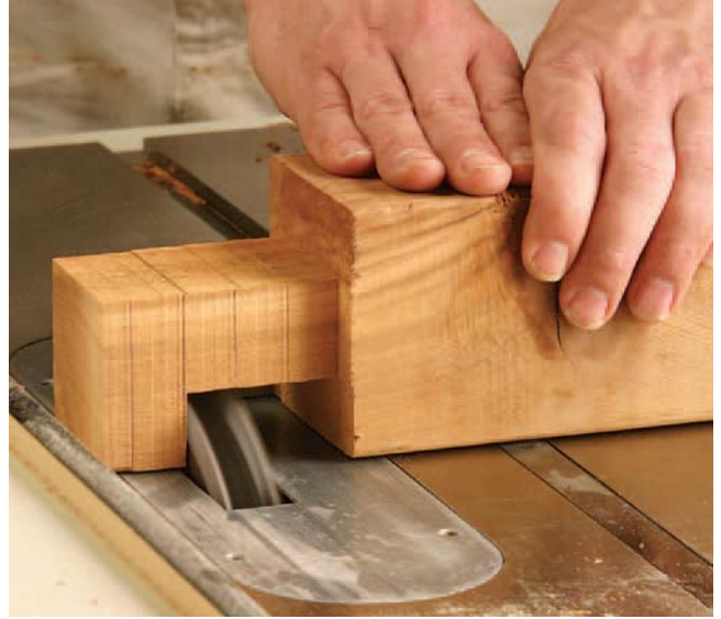
Figure 3: Cut the tenons to thickness with a stacked dado head, machining from both sides of the workpiece to keep the tenon centered. Be sure to start with consistently sized stock.
