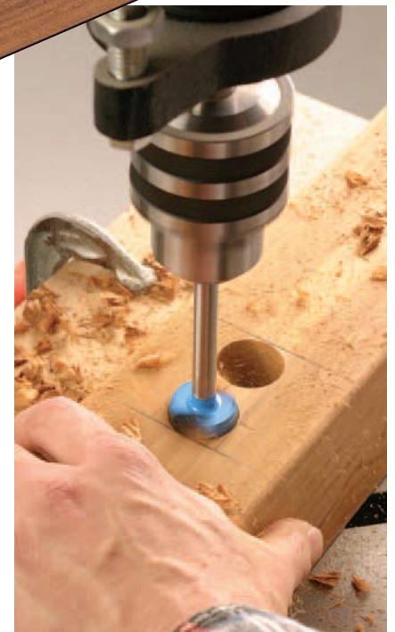
Figure 1: Drill out your mortises with a 1/8" Forstner bit, using a fence to keep the holes aligned in the center of the piece.
