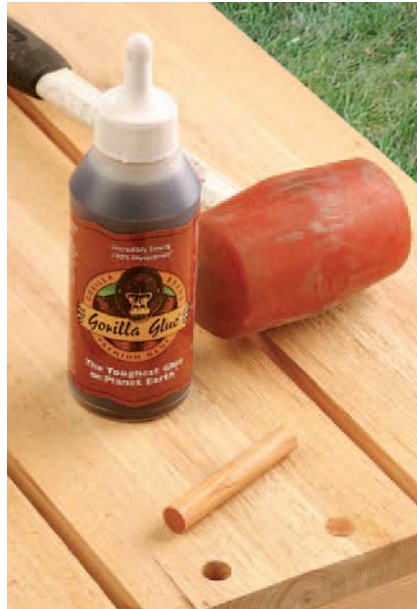
Water-resistant (epoxy and polyurethane) adhesives are excellent choices for building this project. To secure the seat slats, we used 1/2"-diameter hardwood dowels and adhesive to peg the boards in place.
