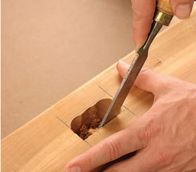
Figure 2: Square up the mortises with a sharp chisel and mallet. The sides of the drilled holes serve as a visual guide.
